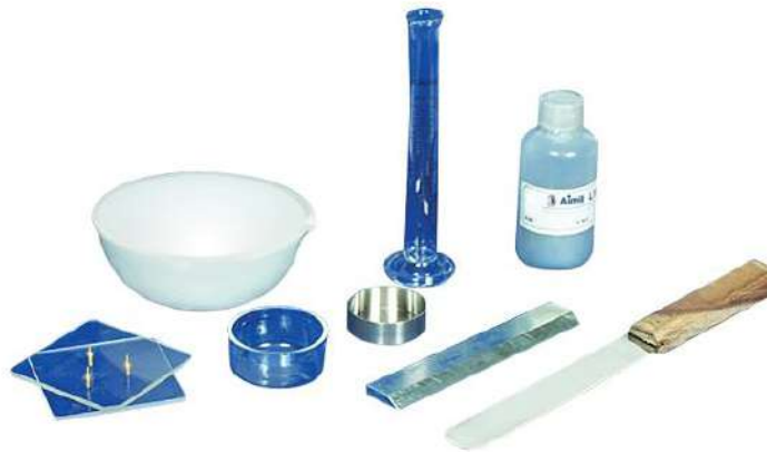
Apparatus required for Shrinkage Limit test
